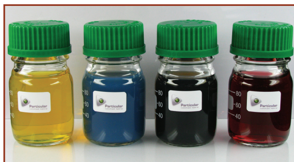
Nanoparticles from metals (silver, titanium, platinum, gold) in water
