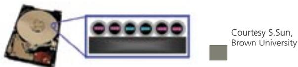
A magnetic hard disk and the schematic illustration of the recorded bits supported by an array of ferromagnetic dots
