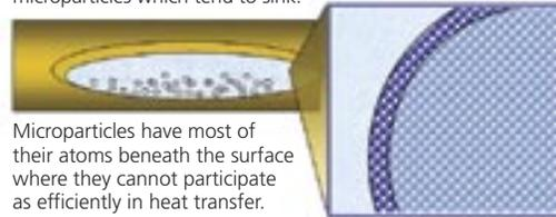
Microparticles have most of their atoms beneath the surface where they cannot participate as efficiently in heat transfer.
