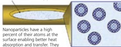
Nanoparticles have a high percent of their atoms at the surface enabling better heat absorption and transfer. They flow more effectively than microparticles which tend to sink.
