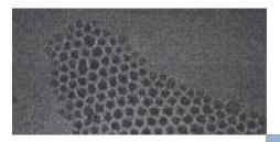
TEM of air stable 10nm Co particles
