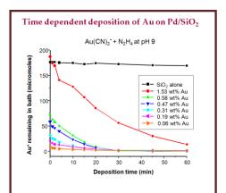
The process is a combination of anodic and cathodic electrochemical partial reactions. The aqueous reducing agent is catalytically activated at the surface of the primary metal to produce an active hydrogen species that reduces the aqueous secondary metal salt on the surface of the primary metal.
