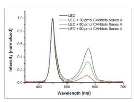
StremDots™ Series A particles modifying a LED spectra
