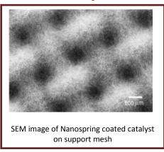
The Nanospring<sup>™</sup> Enzymatic Flow Reactor is a 2.5 inch long, 0.25 inch i.d. tube that is packed with stainless steel mesh coated with a total of approximately 50 mg of silica Nanosprings.
