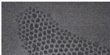
TEM of air stable 10nm Co particles
