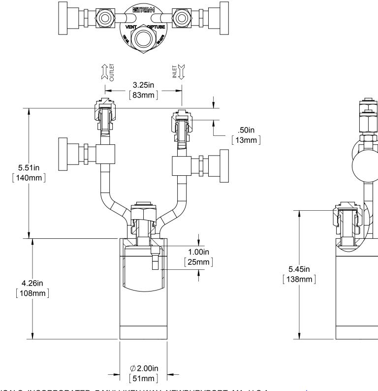
CYLINDER MOD CYLINDER SIZE CYLINDER WOR CYLINDER TOT/ CYLINDER TARE DESIGN PRESS TEST PRESSUR **DESIGN TEMPE** INTERNAL FINIS EXTERNAL FINI FILLPORT INLET VALVE OUTLET VALVE THERMOWELL DIPTUBE MATERIAL OF C D.O.T. SPECIFIC TOLERANCE (UNI
