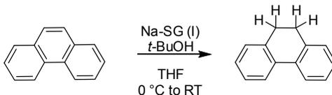
In a typical procedure, phenanthrene and Na-SG(I) are charged into a reactor and stirred under an inert atmosphere. THF is added, and the slurry is cooled to 0 °C. The proton source, *tert*-butanol, is added in one portion and the reaction is allowed to warm to room temperature. The desired product is isolated in 60% yield after an aqueous work-up.
