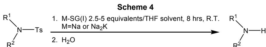
Treatment with M-SG is a mild and general solution process to desulfonate protected amines. Various sulfonamide substrates were investigated. Detosylation with Na<sub>2</sub>K-SG(I) tolerates phenyl and ether moieties and is successful for both cyclic and acyclic amines (Table 3).
