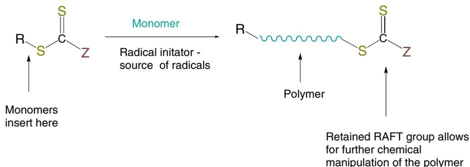
Figure 3: At the heart of it - The process of RAFT polymerization
