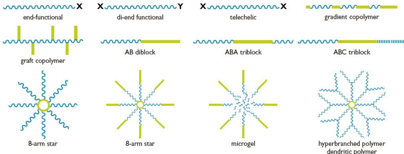
Figure 1: Polymer architectures possible with RAFT technology
