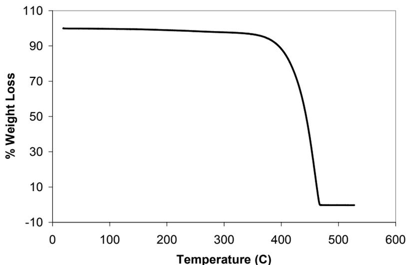
**Figure 2:** Stability with respect to temperature, as demonstrated by thermogravimetric analysis (TGA), for trihexyl(tetradecyl)phosphonium tetrafluoroborate,  $[(C_6H_{13})_3P(C_{14}H_{29})][BF_4]$ .
