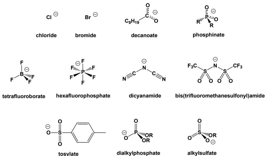
**Figure 1:** Examples of anions that can be paired with tetraalkylphosphonium cations to produce ionic liquids.
